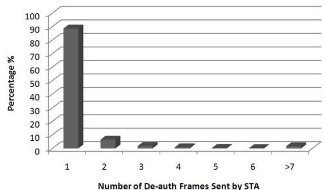
Fig. 2: Percentage distribution of the Number of de-authentication frame(s) sent by clients. possess the ability to automatically re-connect to the same AP if the connection is abruptly terminated in the midst of an ongoing communication. So unless the attacker sustains the attack for an appreciable time, there are high chances that most of the clients recover automatically from the attack and re-connect to the same AP.
